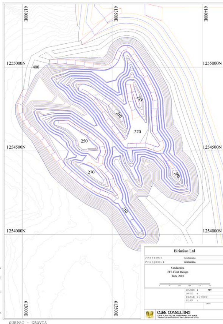
Figure 3: Goulamina PFS Proposed Pit Design
