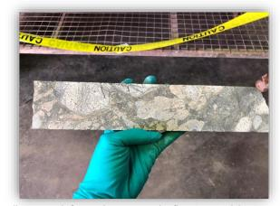
Drill core sample from Nolans Bore used in flotation variability program
