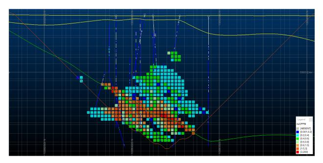
Figure 14-14: Example Cross Section (Looking W) through Tonopah block model (121 Zone). Showing MII blocks and pit trace for reference
