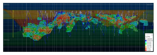
Figure 14-11: Long Section (Looking N20E) view showing drill holes, estimated blocks, and pit shell used to constrain resource estimate. Blocks outside the pit shell are not included in the resource.
