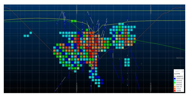
Figure 14-12: Example Cross Section (Looking W) through Tonopah block model (Dauntless Zone). Showing MII blocks and pit trace for reference (Blocks are 20 feet on center)
