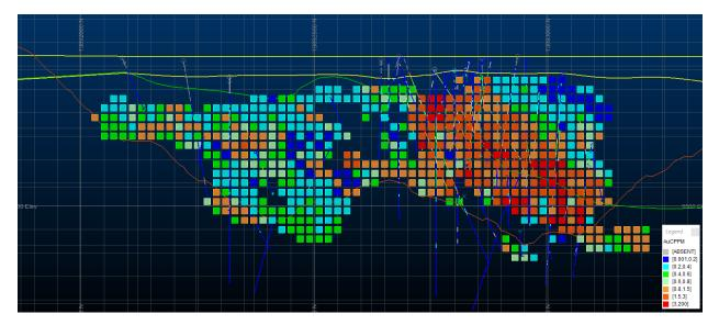
Figure 14-13: Example Cross Section (Looking W) through Tonopah block model (Discovery Zone). Showing MII blocks and pit trace for reference. (Blocks are 20 feet on center)
