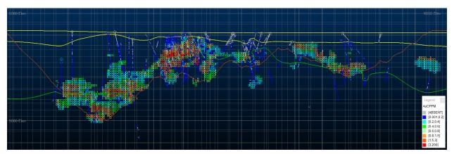
Figure 14-17 Long Section (Looking N20E) showing block grade estimates and pit trace for reference.
