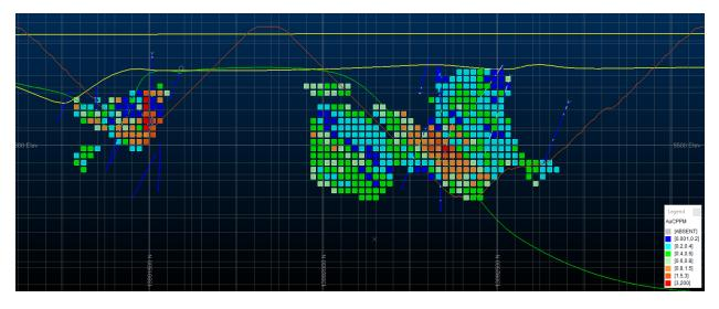
Figure 14-15: Example Cross Section (Looking W) through Enterprise (Left) and 121/Pointluck Zones (right) Showing MII blocks and Pit trace for reference.
