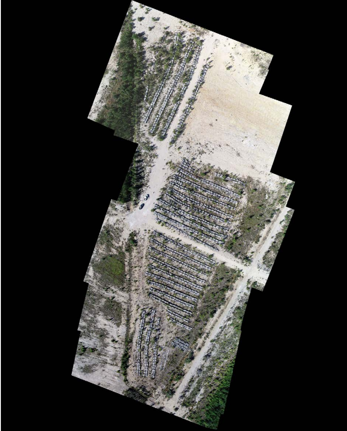
Figure 12-5: An orthomosaic air photo map of the Pine Point core yard (2 F250 trucks for scale centre-left)
