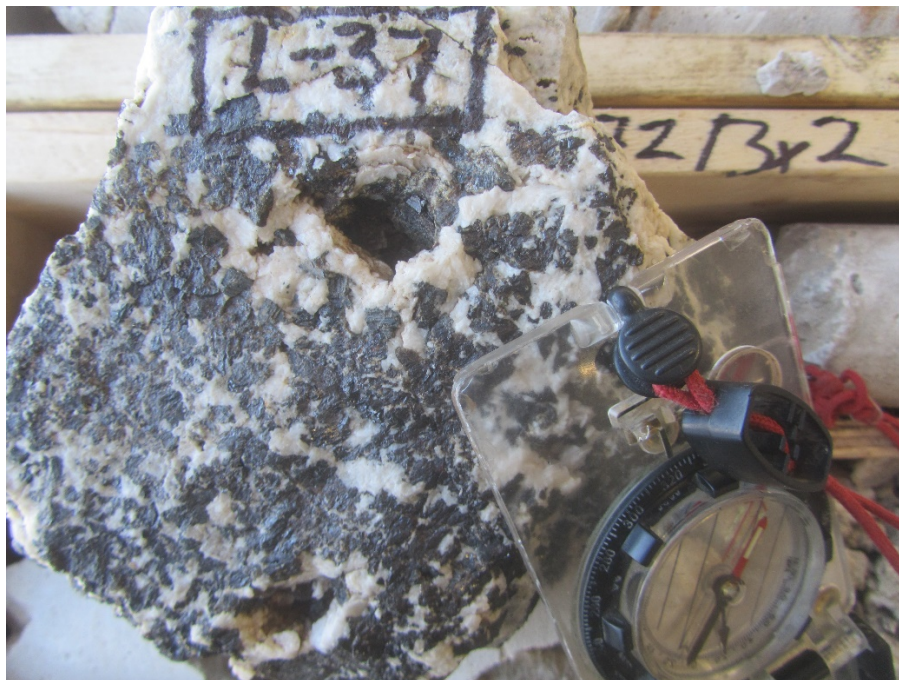
Figure 8-3: Coarse-crystalline sphalerite-rich mineralization at the core of the L37 deposit. Sphalerite crystals up to 10 mm in white 'sparry' dolomite 'gangue'.
