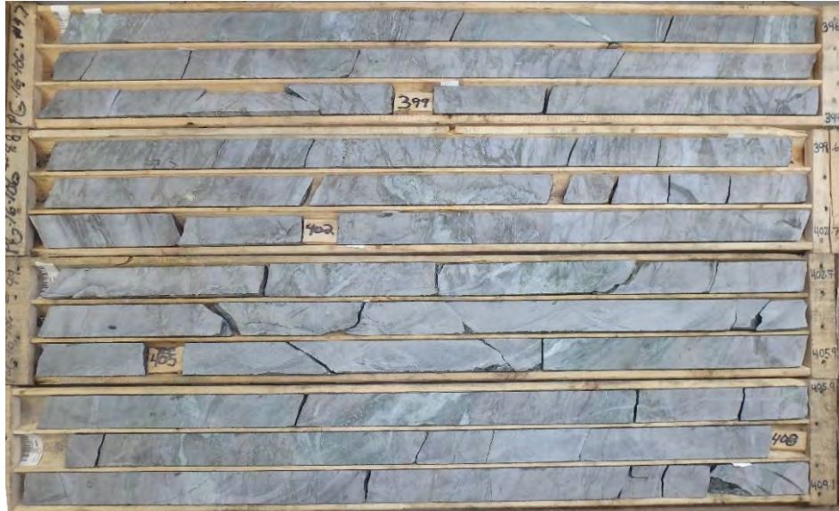
Figure 16-2: Example of Typical Half Core used for Logging and Point Load Testing
