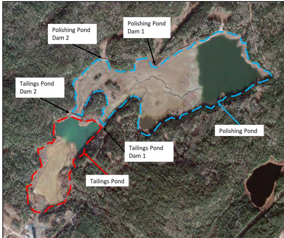
Figure 18-6: Existing TMF General Arrangement
