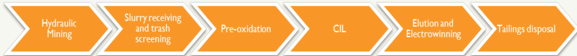
ELIKHULU TAILINGS RE-TREATMENT PLANT FLOW SHEET
