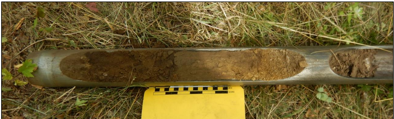
Photo 10-4: Oxidized Tailings Recovered by Percussion Drill on North Perimeter Embankment Cell #2
