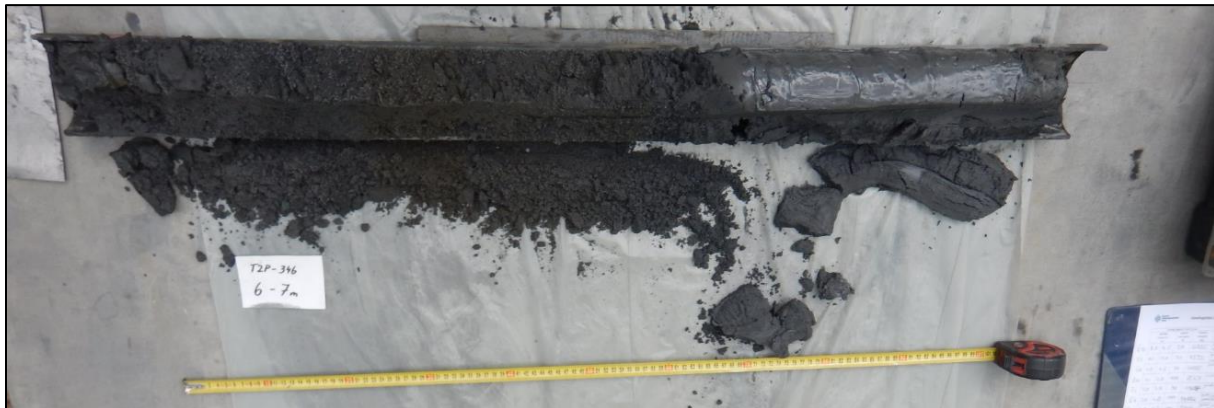
Photo 12-1: View of 1m Tailings Core Being Quarter Split (uphole direction is to right), T2P-346, 6-7m
