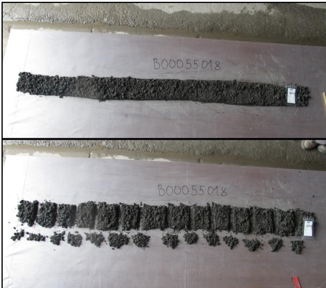
Photo 11-4: Example of Sample Splitting by the Wet Japanese Slab Cake Homogenization Method
