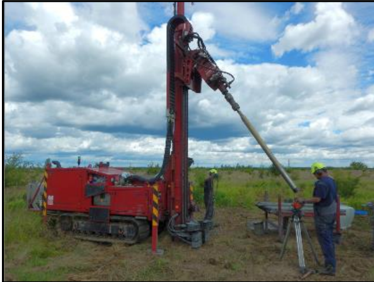
Photo 10-1: Showing Eikelkamp SonicSampDrill B.V. and Drill Crew
