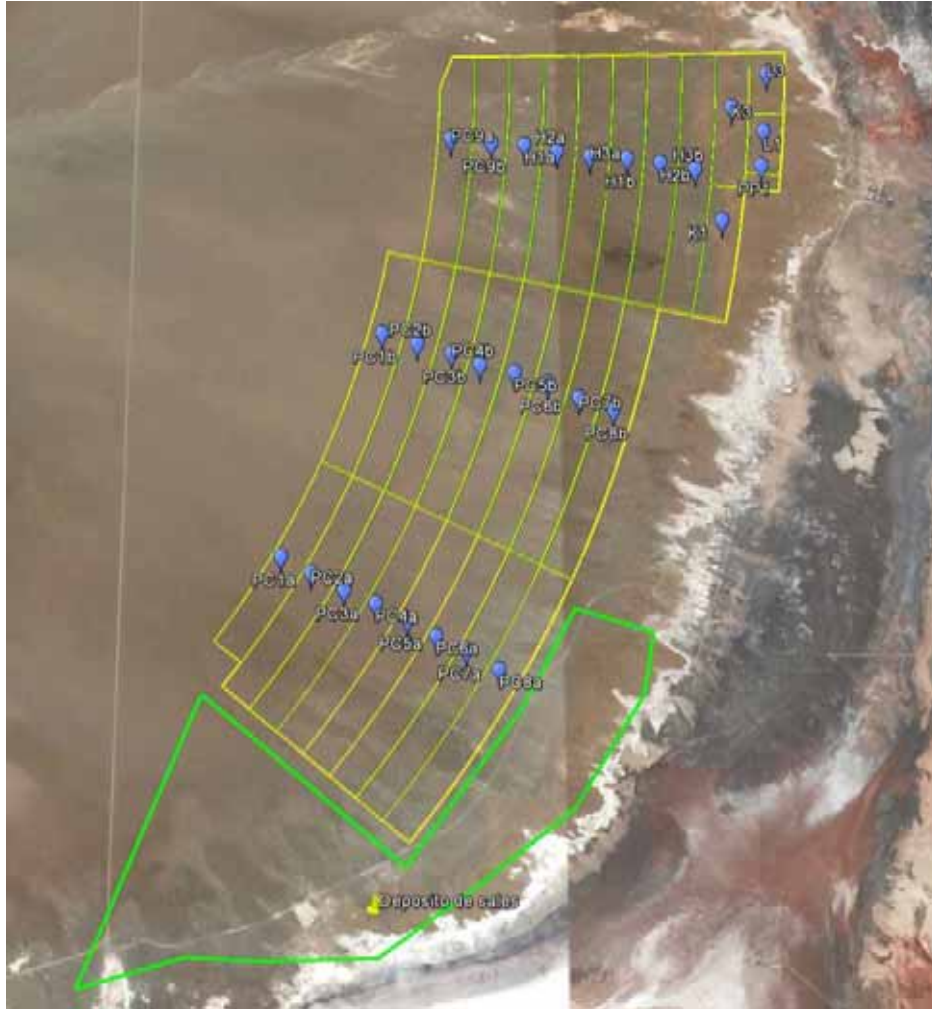
Figure 17.2 Evaporation Ponds and Salt Disposal Area
