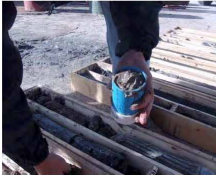
Figure 11.2 Collecting an Undisturbed Sample from Sand Core
