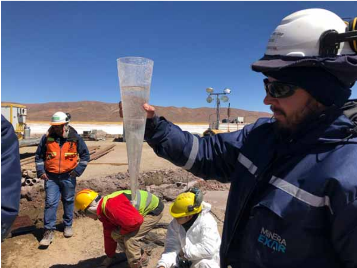
Figure 11.4 Measuring Sediment in an Imhoff Cone
